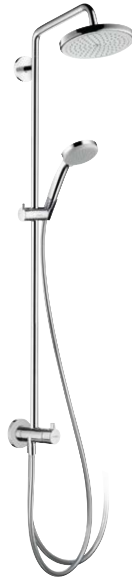
Croma® 220 Air 1jet Showerpipe Reno with swivelling Croma 220 Air 1jet overhead shower (16 l/min), Croma 100 Vario hand shower (15 l/min), without mixer, shower arm 400 mm # 27224, -000 # 27158, -000 Corner installation set (not shown) Height of the Showerpipe can be reduced
