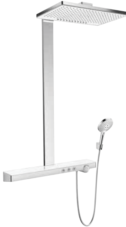
Rainmaker® Select 460 2jet Showerpipe with Rainmaker Select 460 2jet overhead shower (RainXL: approx. 18 l/min; RainStream: approx. 18 l/min), Rairdance Select S 120 3jet hand shower (16 l/min) and ShowerTablet Select 700 thermostat, shower arm 450 mm # 27109, -400 # 27028, -400 EcoSmart (9 l/min)
